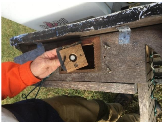
Figure 11. An I-button temperature and humidity logger attached to the inside of a horizontal hardwood Red-rumped Parrot nest box
